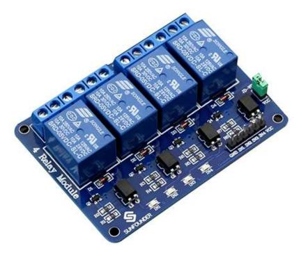
This is a 5V 4-channel relay interface board, and each channel needs a 15-20mA driver current. It can be used to control various appliances and equipment with large current. It is equiped with high-current relays that work under AC250V 10A or DC30V 10A. It has a standard interface that can be controlled directly by microcontroller.
